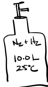
$$\begin{aligned} n_T &= 30.7 \text{ g H}_2 \times \frac{1 \text{ mole H}_2}{2.016 \text{ g H}_2} + 1.62 \text{ g N}_2 \times \frac{1 \text{ mole N}_2}{28.02 \text{ g N}_2} \\ &= 15.2817 \text{ mole H}_2 + 0.057816 \text{ mole N}_2 \end{aligned}$$
