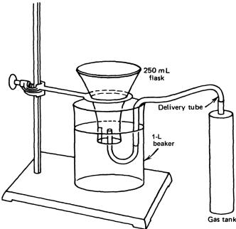
Figure 19.1 Apparatus for collecting gas samples
